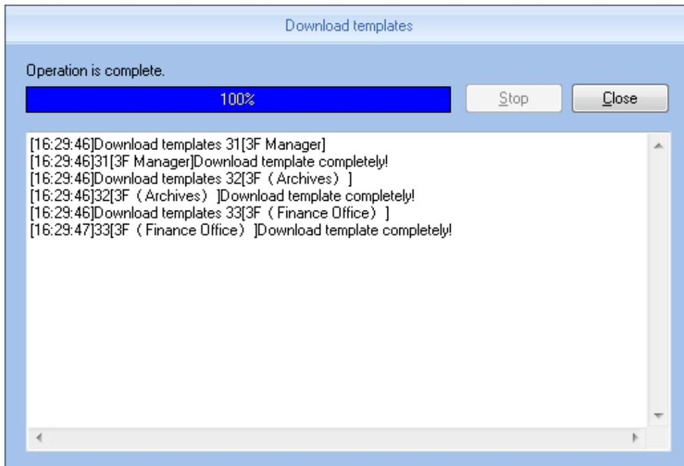
After download template is finished, you can see the column of download template fill color. That means the fingerprint has been downloaded.
