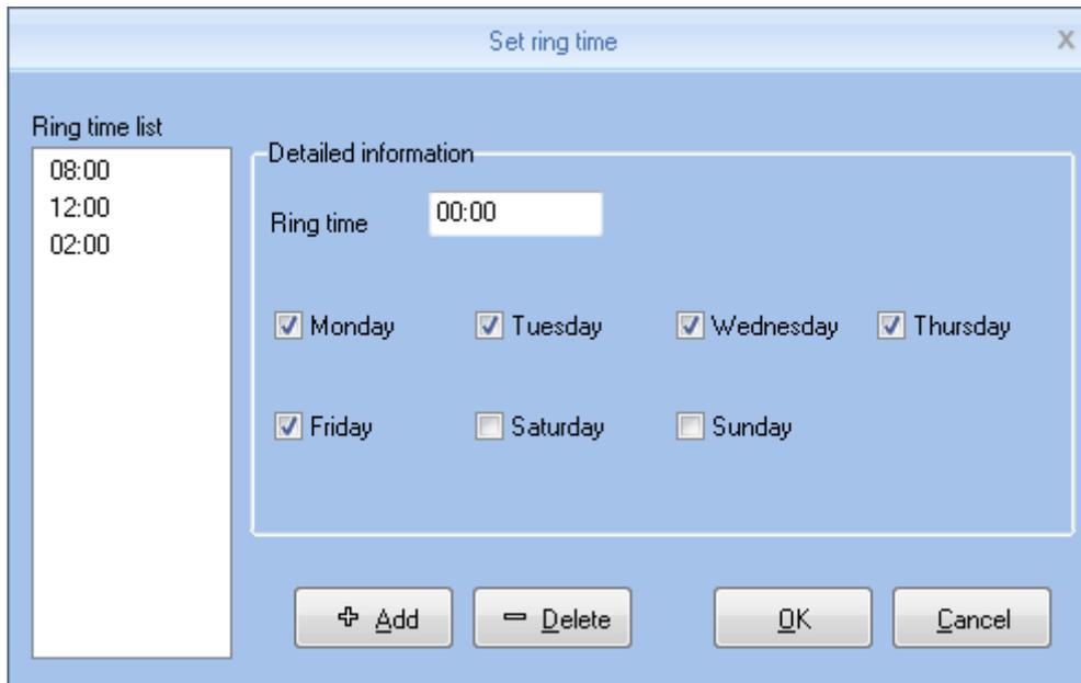
Set the desired time bell rang the bell at the time of the entry box. Click [+ Increases (A)] button to add time to time list. When the time list for invalid bell time, you can delete the invalid time. Select delete bell time, click - [Delete (D)] button to bring up the dialog box to confirm the deletion:
