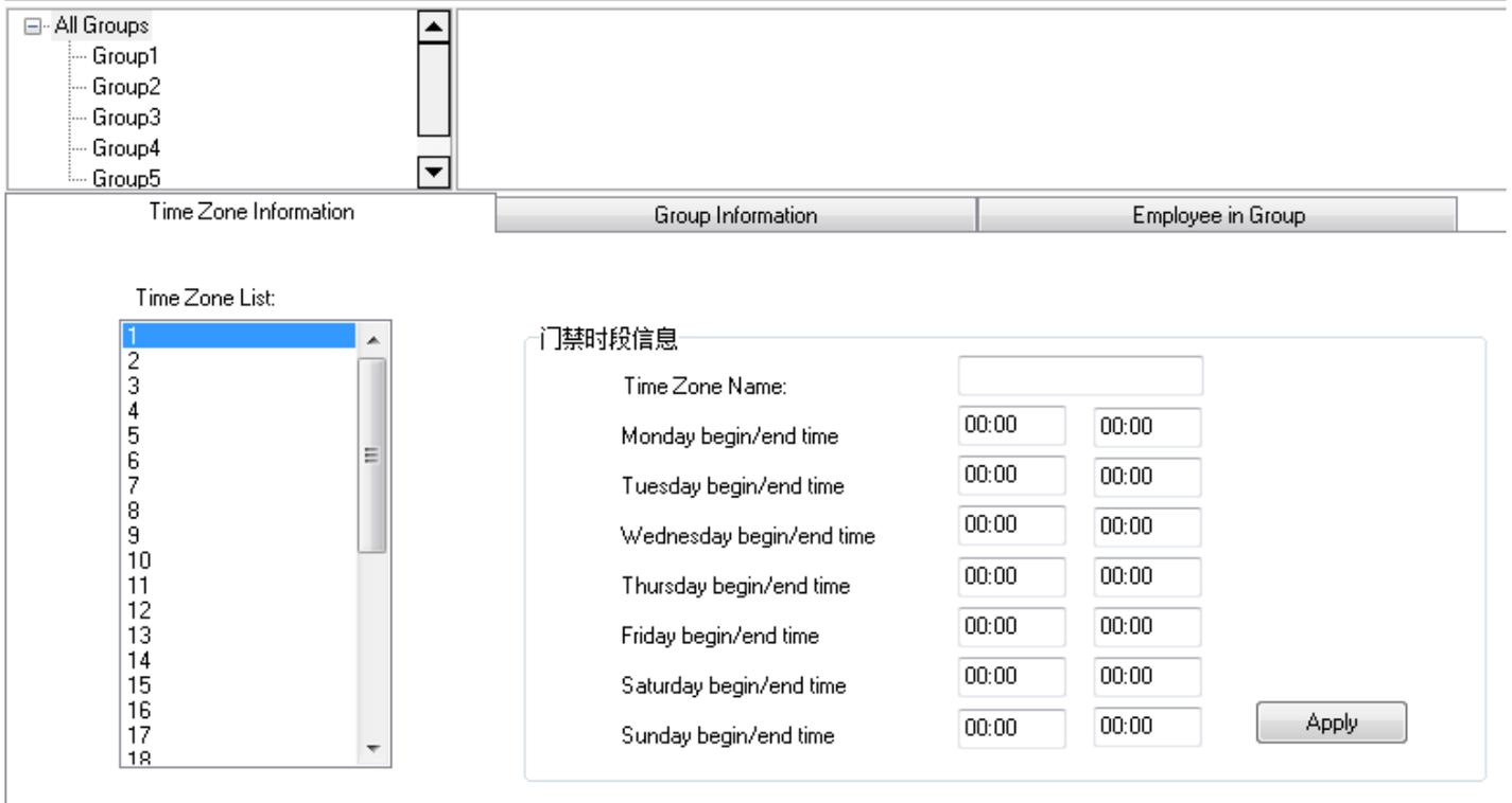
Anviz crosschex software support 32 access control timetable and 16 access control group, one group support 4 timetables, the target is to setup access timetable to staff, and connect all timetable to a access rule, and give rights to the according staff.
